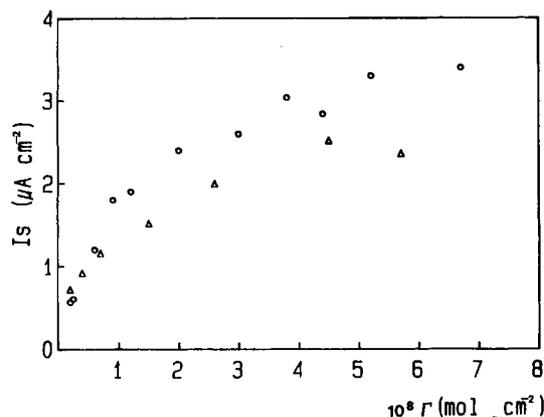
**Figure 2.** Plots of the steady-state photocurrents  $I_s$  vs poly(PMV<sup>2+</sup>) (O) and poly(PPV<sup>2+</sup>) (Δ) thickness.  $[(C_6H_5)_2C(OH)CO_2^-] = 5 \times 10^{-2}$  M in both cases.
