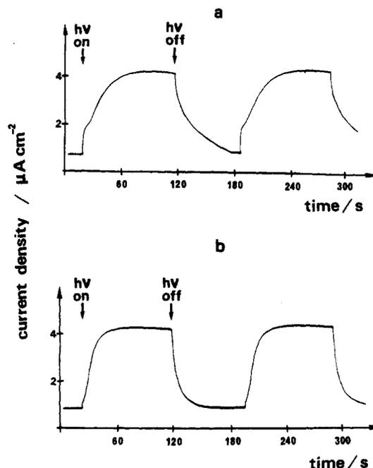
Figure 1. Photocurrent responses of an OTE coated with (a) a poly(PPV<sup>2+</sup>) film ( $\Gamma = 4.5 \times 10^{-8}$  mol cm<sup>-2</sup>); (b) a poly(PMV<sup>2+</sup>) film ( $\Gamma = 5.2 \times 10^{-8}$  mol cm<sup>-2</sup>) in the presence of (C<sub>6</sub>H<sub>5</sub>)<sub>2</sub>C(OH)CO<sub>2</sub><sup>-</sup> ( $C = 5 \times 10^{-3}$  M) in CH<sub>3</sub>CN + 0.1 M TEAP solution.
