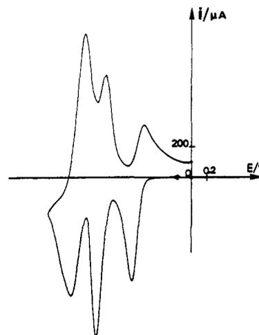
**Figure 8.** Cyclic voltammetry of an OTE/poly(PMV<sup>2+</sup>) (Γ = 2.6 × 10<sup>-8</sup> mol cm<sup>-2</sup>), poly(PNB) (Γ = 5.8 × 10<sup>-8</sup> mol cm<sup>-2</sup>) copolymer film in CH<sub>3</sub>CN + 0.1 M TEAP solution; scan rate ν = 0.05 V s<sup>-1</sup>.
