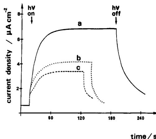
**Figure 3.** Photocurrent responses of an OTE coated with (a) a poly(PV<sup>2+</sup>PTZ) film ( $\Gamma = 2 \times 10^{-8}$  mol  $cm^{-2}$ ); (b) a poly(PV<sup>2+</sup>TPA) film ( $\Gamma = 2 \times 10^{-8}$  mol  $cm^{-2}$ ); (c) a poly(PV<sup>2+</sup>BZ) film ( $\Gamma = 2 \times 10^{-8}$  mol  $cm^{-2}$ ) with  $(C_6H_5)_2C(OH)CO_2^-$  ( $C = 5 \times 10^{-2}$  M) in  $CH_3CN + 0.1$  M TEAP solution.
