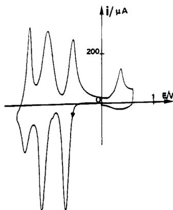
**Figure 5.** Cyclic voltammogram of a Pt electrode modified by a film of poly(PV<sup>2+</sup>NB) ( $\Gamma = 3.7 \times 10^{-8}$  mol cm<sup>-2</sup>) in CH<sub>3</sub>CN + 0.1 M TEAP solution; scan rate  $\nu = 0.1$  V s<sup>-1</sup>.
