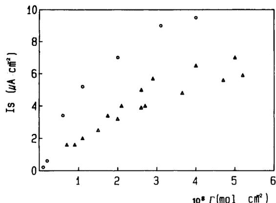
**Figure 4.** Plots of the steady-state photocurrent  $I_s$  vs poly(PV<sup>2+</sup>PTZ) (O), poly(PV<sup>2+</sup>BZ) (Δ) and poly(PV<sup>2+</sup>TPA) (Δ) thickness. [(C<sub>6</sub>H<sub>5</sub>)<sub>2</sub>C(OH)CO<sub>2</sub><sup>-</sup>] = 5 × 10<sup>-2</sup> M in all cases.
