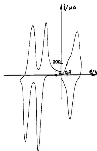
**Figure 7.** Cyclic voltammetry of an OTE/poly(PMV<sup>2+</sup>) ( $\Gamma = 5 \times 10^{-8}$  mol cm<sup>-2</sup>)/poly(PPTZ) ( $\Gamma = 3.6 \times 10^{-8}$  mol cm<sup>-2</sup>) bilayer in CH<sub>3</sub>CN + 0.1 M TEAP solution; scan rate  $\nu = 0.05$  V s<sup>-1</sup>.
