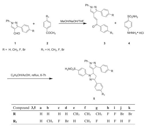
Scheme 1. Synthesis of 5a-5k from formylpyrazoles (1).
