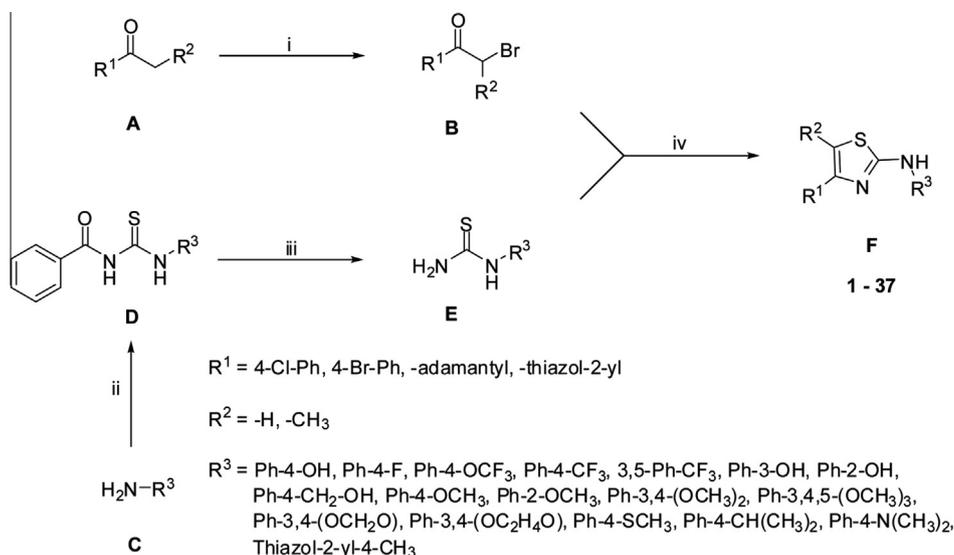
**Scheme 1.** General procedure for the synthesis of 2-aminothiazole derivatives **1–37**. Reagents and conditions: (i)  $\text{Br}_2$ , chloroform, rt, 2 h; (ii) benzoyl chloride,  $\text{NH}_4\text{SCN}$ , acetone,  $60^\circ\text{C}$ , 45 min; (iii)  $\text{NaOH}$  (2 M),  $\text{H}_2\text{O/THF}$ ,  $100^\circ\text{C}$ , 1 h; (iv) ethanol, microwave irradiation,  $80^\circ\text{C}$ , 30 min.
