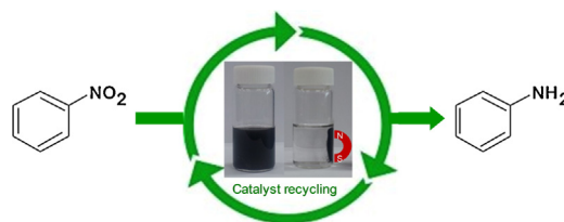
Fig. 6. Magnetic separation and recycling of the carbon nanocomposite Pt catalyst.
