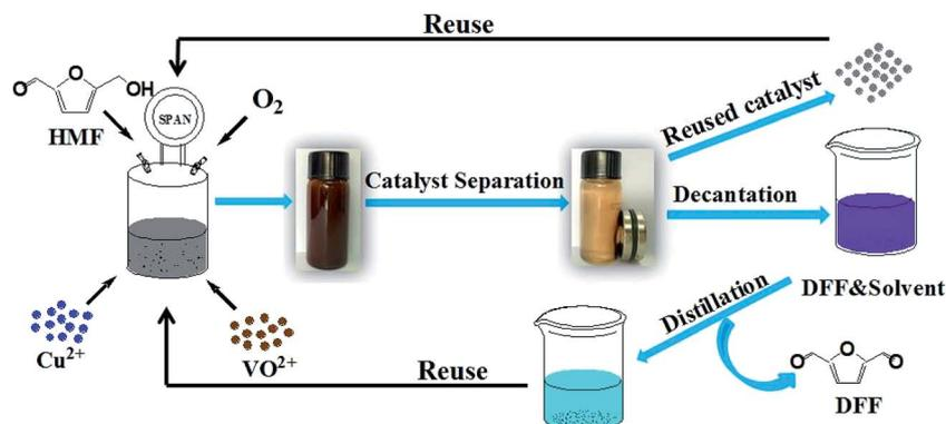
Scheme 4 The schematic illustration of procedures for recycling of catalysts and solvent.
