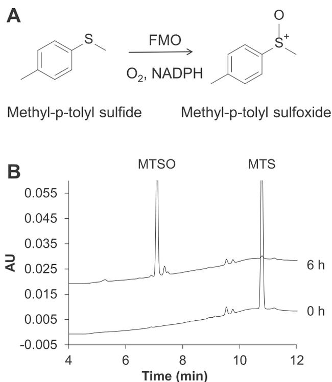
**Fig. 2.** S-oxygenation potential of the human FMO4 transformant towards methyl-p-tolyl sulfide. (a) Reaction scheme of MTS S-oxygenation. (b) HPLC profile of 0.1 mM MTS incubated with the FMO4 transformant for 0 and 6 h.
