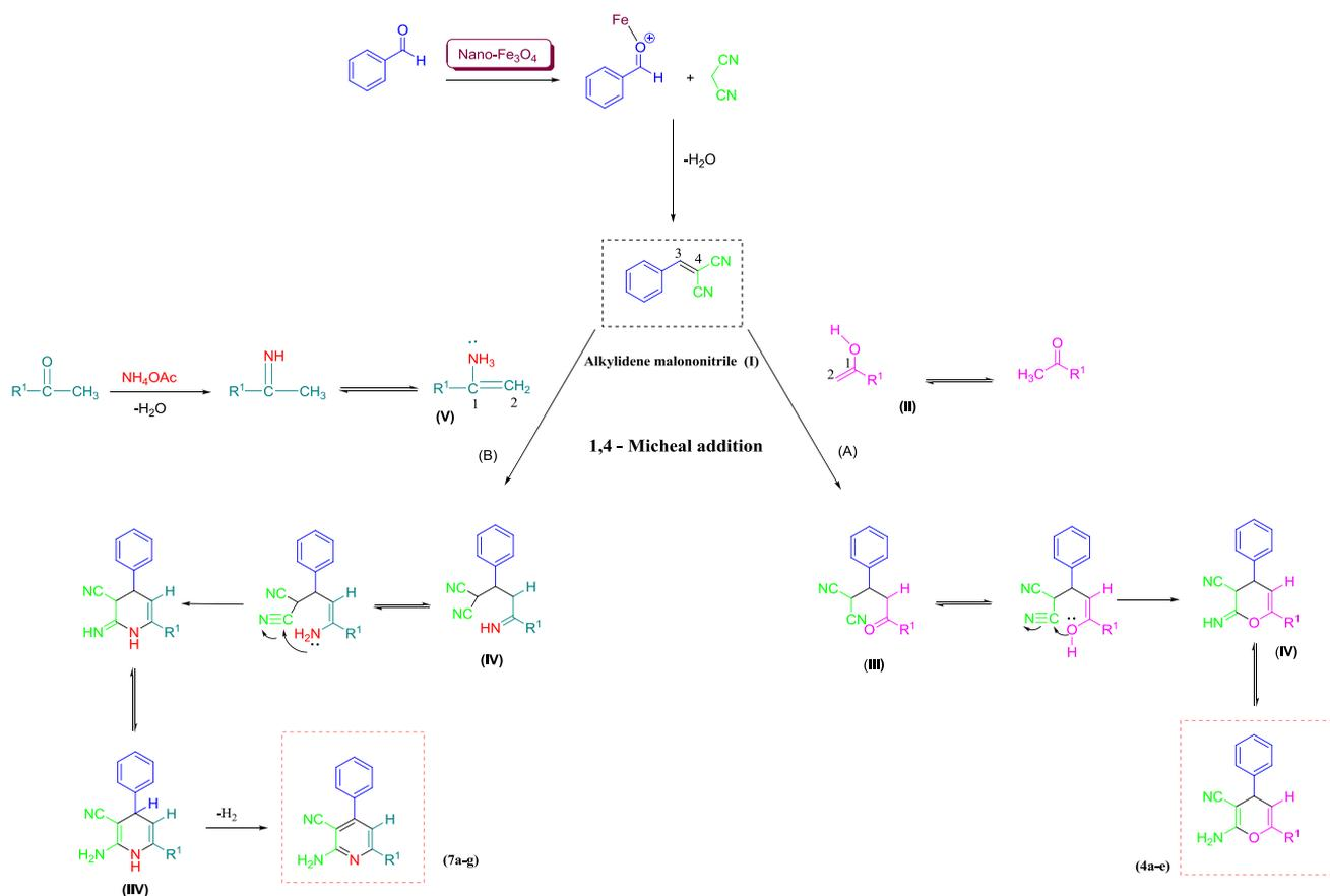
**Scheme 3** Proposed mechanism of the synthesis of (**4a–e**), (**7a–g**)
