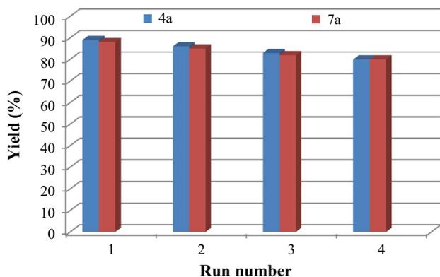
**Fig. 1** The recyclability of the  $\text{Fe}_3\text{O}_4$  in the preparation of **4a** and **7a**
