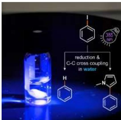
**Photoredox catalysis takes a bath:** Single-chain polymeric nanoparticles are utilized as an efficient and recyclable platform to perform photoredox catalysis in water. The reduction of aryl halides and C-C cross coupling reactions are studied upon UV light illumination at ambient conditions.
