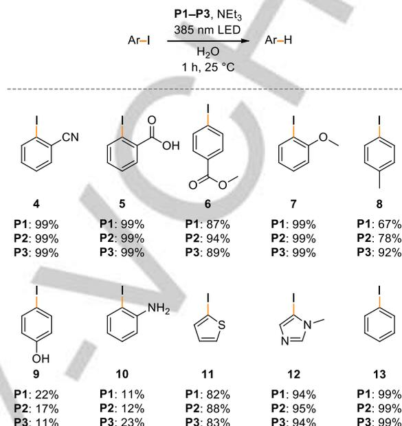
**Scheme 1.** Illustration of the reaction scope for the dehalogenation of differently substituted (hetero)aryl iodides. The indicated conversions are average results of at least two experiments following the general protocol. The reduction of 2-iodobenzoic acid **5** was carried out in deuterated water.
