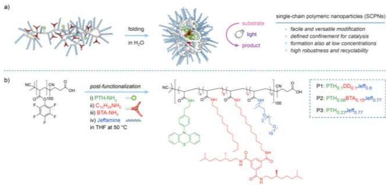
**Figure 1.** Photoredox-active single-chain polymeric nanoparticles: a) Illustration of the intramolecular hydrophobic collapse of an individual chain to a nanoparticle in water, furnishing an apolar interior as platform for photoredox catalysis. b) Post-functionalization of poly(pentafluorophenyl) acrylate by the sequential addition of amine-bearing compounds to yield the catalytically active polymers **P1–P3**.
