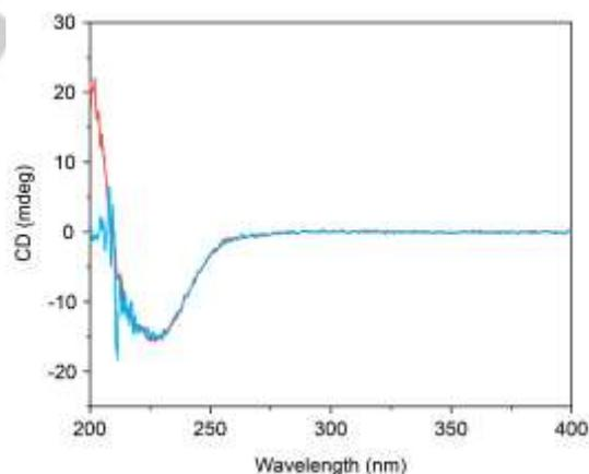
**Figure 3.** CD spectra of a solution of **P2** in water ( $c = 0.1$  mg/mL,  $V = 3$  mL) before (red curve) and after the addition of 1 μL of triethylamine (ca. 2300 eq., blue curve) at 20 °C. The negative CD signal, which originates from supramolecular helical stacks of the BTA units<sup>[41,53]</sup> within the nanoparticles' core, is not affected by the presence of triethylamine.
