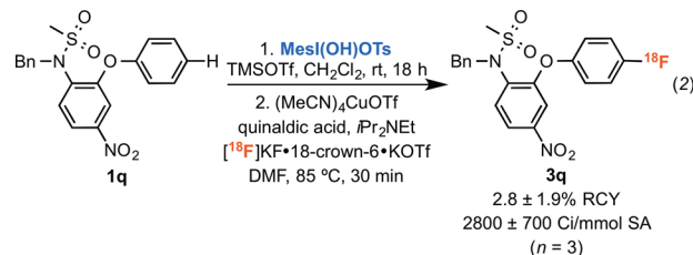
Figure 1. Cu-mediated C(sp 2 )–H radiofluorination of electron-rich arenes. Conditions: (1) 1 (10 μmol), MesI(OH)OTs (10 μmol), TMSOTf (10 μmol), CH 2 Cl 2 (40 μL); (2) (MeCN) 4 CuOTf (10 μmol), quinaldic acid (10 μmol), i Pr 2 NEt (20 μmol), [ 18 F]KF·18-crown-6·K 2 CO 3 complex in DMF (100 μL, 80–1200 μCi), total volume 1.0 mL. Reported radiochemical conversions were measured by radio-TLC (average of n runs) and were corrected for presence of 4 (ratio of 3/4 determined by radio-HPLC). The identity of each product was confirmed by radio-HPLC. Key: (a) 105 °C; (b) TMSOTf (5 μmol). 25,26
