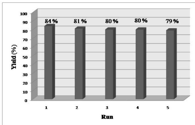
**Figure 2.** Study of reusability SSA in cyanation of 3-methylphenol.
