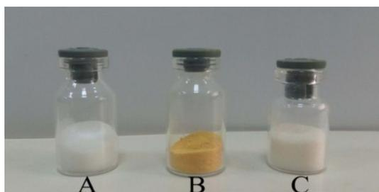
**Figure 3.** The color of SSA before (A) and after the reaction (B) and after recovery process (C).
