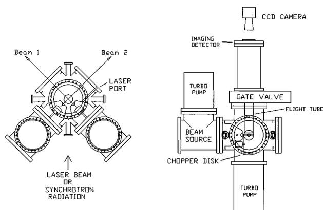
FIG. 1. Schematic view of “universal imaging” machine. Left view is from above, right view is into the primary beam source.
