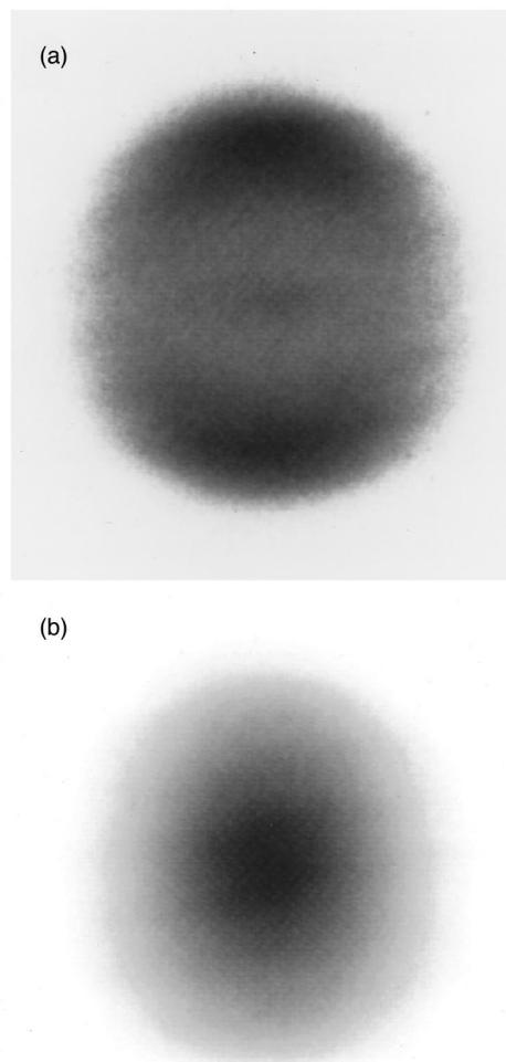
FIG. 2. (a). Raw image of  $\text{Cl}^*(^2P_{1/2})$  recorded with dissociation and probe at 235.205 nm on the  $4p^2P_{1/2} \leftarrow 3p^2P_{1/2}$  transition. (b) Raw image of  $\text{Cl}(^2P_{3/2})$  recorded with dissociation and probe at 235.336 nm on the  $4p^2D_{3/2} \leftarrow 3p^2P_{1/2}$  transition. The laser polarization direction is vertical in the plane of the images.
