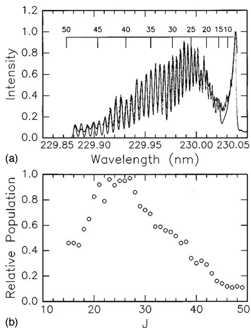
FIG. 5. (a) REMPI scan of CO  $v=0$  on the  $B \leftarrow X$  transition obtained as described in text (+), along with simulation (solid line). (b) Rotational population obtained from the simulation above.
