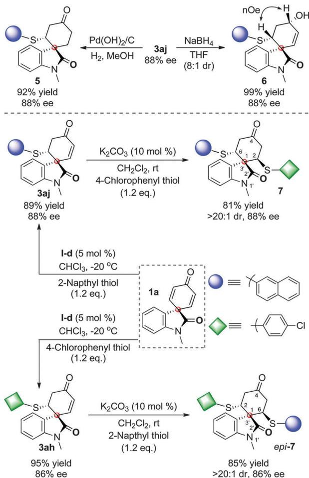
Scheme 2 Synthetic transformation and synthesis of compounds **7** and *epi-7* via double SMA by switching the adding sequence of thiols.
