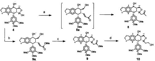
Reagents & Conditions : (a) PPh3=CHCOMe, toluene, pyridine, 90°C, 3h,80%; (b) PPh3=CHCOOMe, toluene, pyridine, 90°C, 3h, 70%; (c) Toluene, NEt3, 100°C, 80%; (d) Lithum aluminium hydride, THF, 0°C, 1h, 80%;
