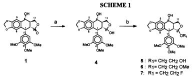
**Reagents & Conditions :** (a) 1.0M soln of disobutylaluminiumhydride in toluene, DCM,  $-70^{\circ}$ C, 40min., 70%; (b) Ethylene glycol for 5, 2-methoxyethanol for 6, 2-fluoroethanol for 7, 1,2-dichloroethane, *p*-toluenesulfonic acid, 25°C, 30min., 60-70%;
