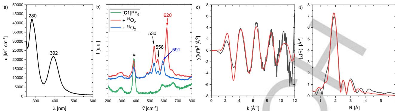
**Figure 1.** a) UV/Vis spectrum of **[O1](PF<sub>6</sub>)<sub>2</sub>** (0.5 mM) in THF at  $-90\text{ }^{\circ}\text{C}$ . b) resonance Raman spectra of **[O1](PF<sub>6</sub>)<sub>2</sub>** in THF with excitation at 420 nm (blue:  $^{18}\text{O}_2$ , red:  $^{16}\text{O}_2$ , green: **[C1]PF<sub>6</sub>**, #: solvent), c)  $k^3$ -weighted Cu-K-edge EXAFS of **[O1](PF<sub>6</sub>)<sub>2</sub>**, d) phase-corrected Cu-K-edge Fourier transform of EXAFS of **[O1](PF<sub>6</sub>)<sub>2</sub>**.
