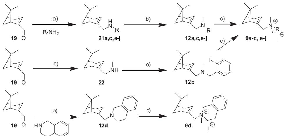
**Scheme 2.** Synthesis of compounds with varying aromatic groups. Reagents and conditions: (a) NaBH(OAc)<sub>3</sub>, DCE, (TEA), rt, 1–2 d; (b) HCOOH, 37% aq. H<sub>2</sub>CO, 2–4 h, reflux; (c) [1] DCM, MeI, 1–3 d, rt [2] DCM/*t*BuOMe, 0 °C, filtration. (d) [1] H<sub>2</sub>NMe (33% in EtOH), MeOH, 1 d, rt [2] NaBH<sub>4</sub>, 3 h, rt, 89%. (e) NaBH(OAc)<sub>3</sub>, 2-iodobenzaldehyde, DCE, rt, 20 h, 36%.
