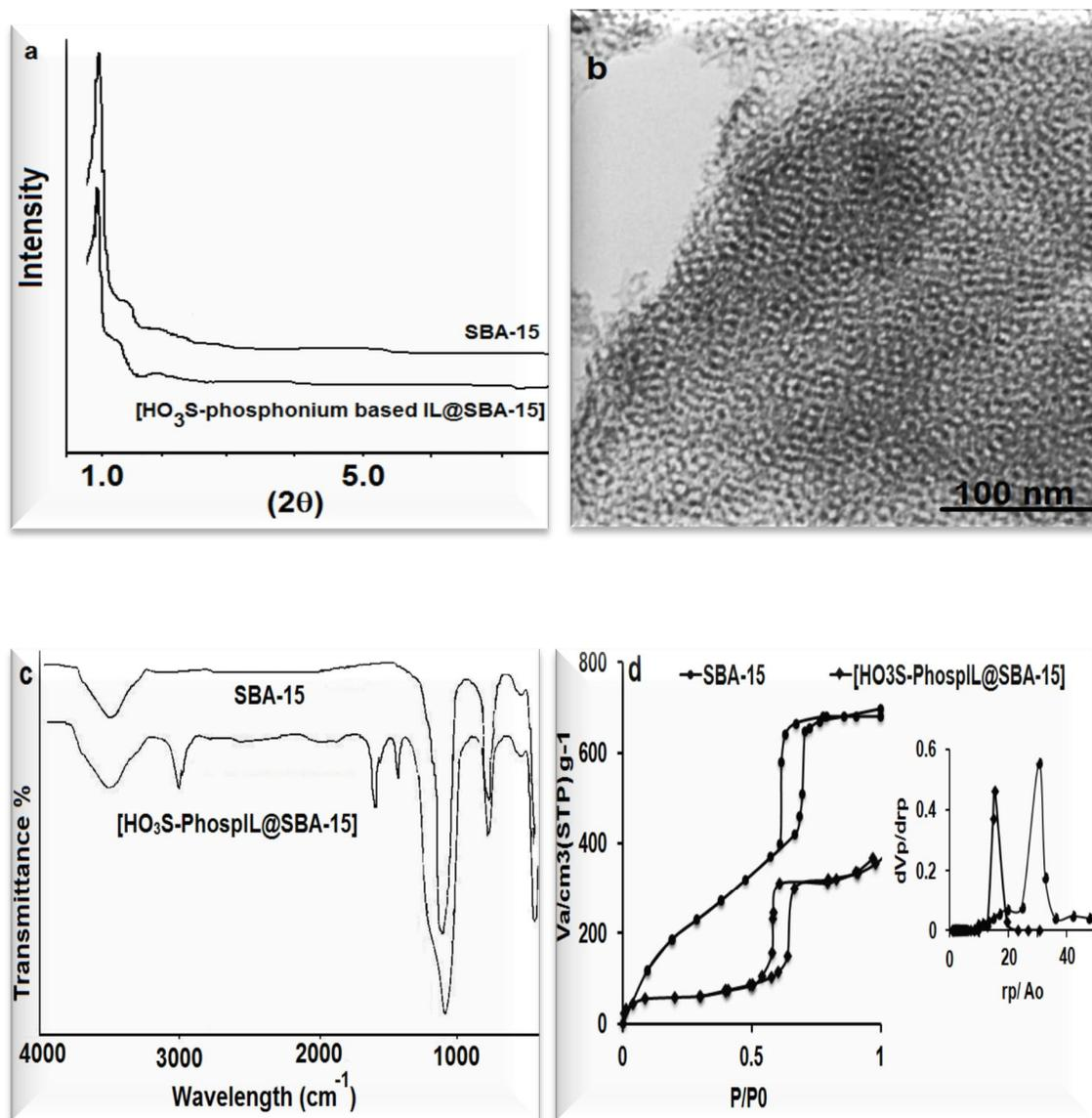
Fig. 1. XRD pattern (a), TEM (b), FTIR spectra (c), and N<sub>2</sub> adsorption-desorption analysis of SBA-15 and [HO<sub>3</sub>S-PhospIL@SBA-15].
