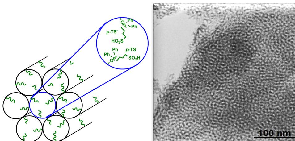
Fig. 2. Sulfonic acid supported phosphonium based ionic liquid functionalized SBA-15 [HO<sub>3</sub>S-PhospIL@SBA-15].
