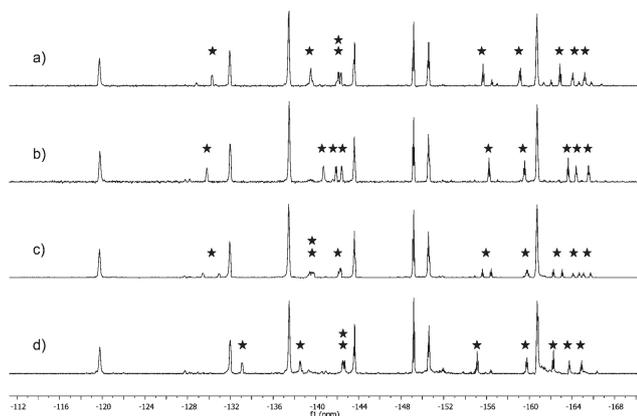
**Fig. 2**  $^{19}\text{F}$  NMR spectra showing formation of  $[\text{HPBB}]^-$  resonances ( $\star$ ) of (a) **4** after heating at  $90^\circ\text{C}$  for 24 h, (b) **6** after heating at  $90^\circ\text{C}$  for 24 h, (c) **5** after 24 h at  $20^\circ\text{C}$ , and (d) **5** after heating at  $90^\circ\text{C}$  for 3 days. Unlabelled resonances correspond to unreacted PBB.
