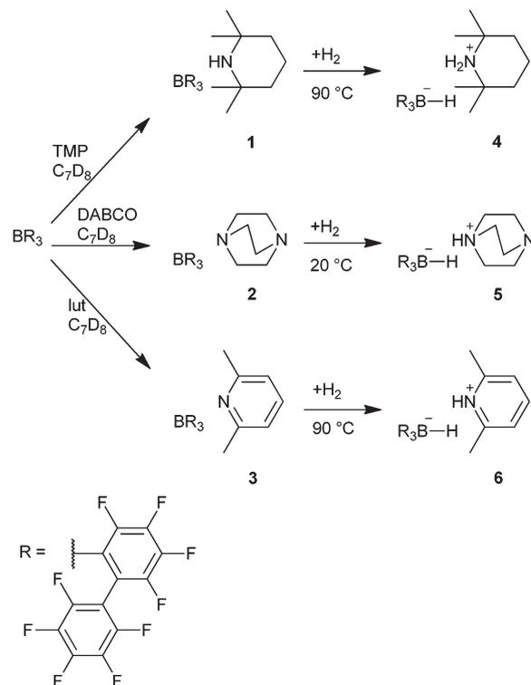
**Scheme 1** Reactions of tris(2,2',2''-perfluorobiphenyl)borane with nitrogen bases and dihydrogen.
