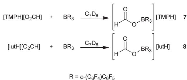
**Scheme 2** Reaction scheme showing the formation of the boroformate salts  $[\text{TMPH}][\text{HCO}_2\text{PBB}]$ , (**7**) and  $[\text{lutH}][\text{HCO}_2\text{PBB}]$ , (**8**).
