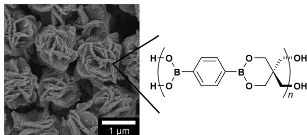
Fig. 1 FE-SEM image of boronate particles (BPs).
