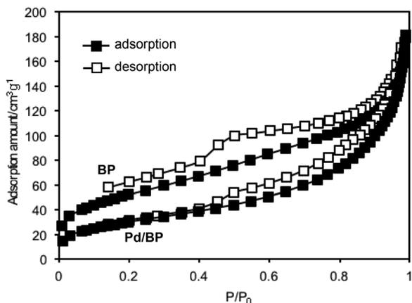
Fig. 3  $N_2$  adsorption–desorption isotherms of BP and Pd/BP.
