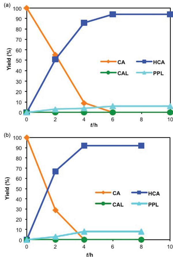
Fig. 4 Hydrogenation of CA (0.3 mmol) in H $_2$ O (a) and MeOH (b) at 25 °C and 0.1 MPa in the presence of Pd/BP (Pd; 0.5 mol%).
