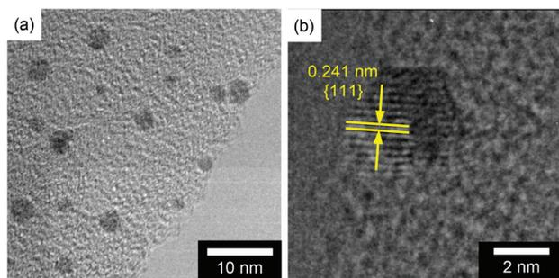
Fig. 5 (a) TEM image of Au/BP. (b) HR-TEM image of a lattice structure observed for the {111} facet of the Au NPs.
