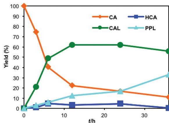
Fig. 6 Amount of CA, HCA, CAL, and PPL as a function of time in the hydrogenation of CA over Au/BP (Au: 1.1 mol%) in H<sub>2</sub>O at 0.8 MPa H<sub>2</sub> and 80 °C.
