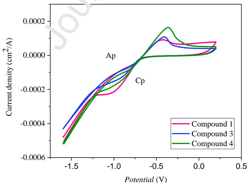
Fig. 10. Cyclic voltammogram of compounds **1**, **3** and **4** ( $1 \times 10^{-4}$   $\mu\text{M}$ ) obtained using a working electrode. The compounds **1**, **3** and **4** were dissolved in DMSO. Ap (anodic process) and Cp (cathodic process). Scan rate:  $0.1 \text{ V s}^{-1}$ .
