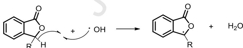
Fig. 12. Reaction between isobenzofuranone and hydroxyl radical with formation of isobenzofuranonyl radicals.
