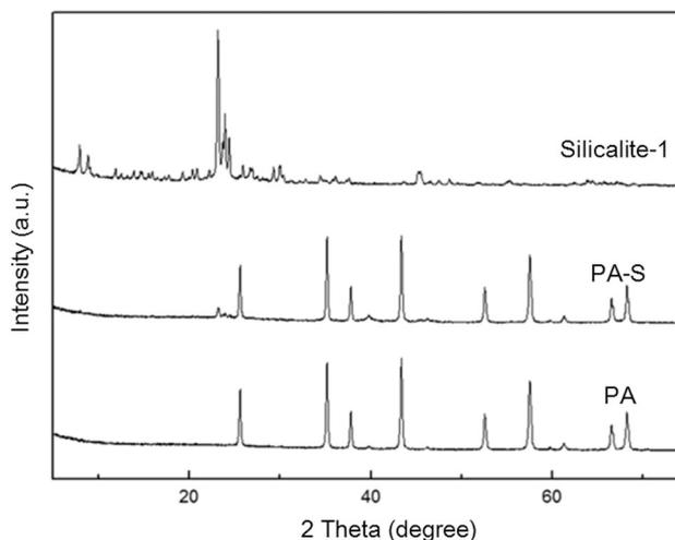
Fig. 1. XRD patterns of PA-S, PA and pure silicalite-1.
