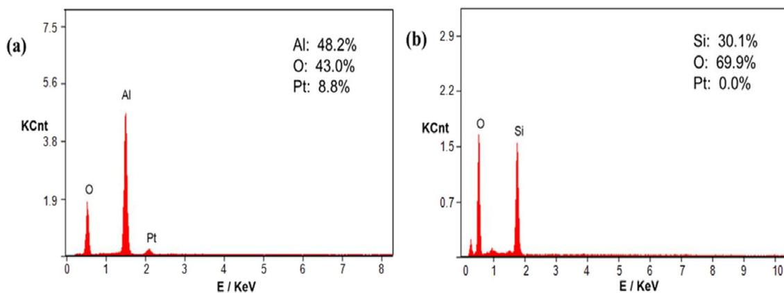
**Fig. 3.** Surface EDS analysis of (a) the bare PA catalyst and (b) the PA-S core-shell catalyst.
