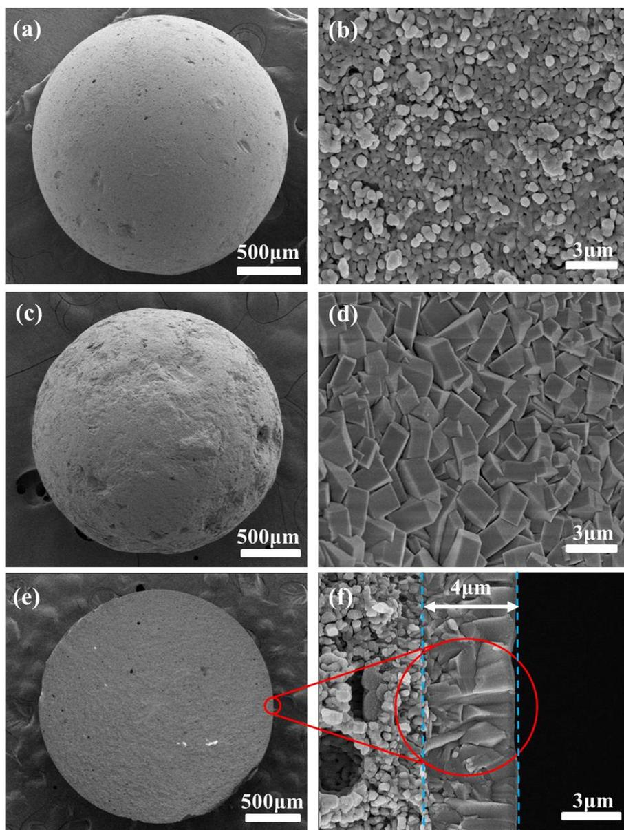
**Fig. 2.** (a, b) Top-view SEM images of the PA catalyst, (c, d) top-view SEM images and (e, f) cross-section SEM images of the PA-S core-shell catalyst under low (left) and high (right) magnifications.
