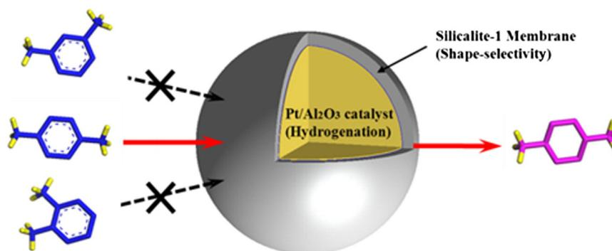
**Scheme 1.** Selective hydrogenation model of xylene isomers over the PA-S core-shell catalyst.
