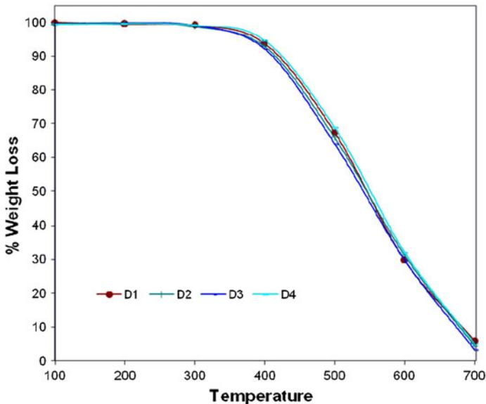
**Fig. 6** Thermogram of the PIs (**D**<sub>1–4</sub>)
