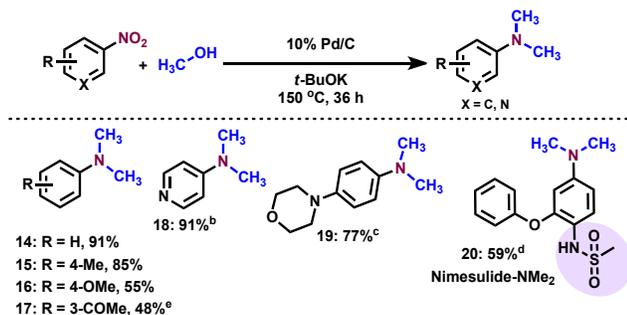
**Scheme 4.** Pd/C-catalyzed *N,N*-dimethylation of nitroaromatics with MeOH.<sup>[a]</sup> Reaction conditions: 0.5 mmol of nitroarene, 10% Pd/C (4.7 mol% Pd, 25 mg), 2 ml of MeOH as a reagent and solvent, *t*-BuOK (2 mmol, 4 equiv.), 36 h, 150 °C, isolated yields. <sup>b</sup> 48 h. <sup>c</sup> 30 h. <sup>d</sup> 60 h. <sup>e</sup> Pd/C (60 mg), *t*-BuOK (2 mmol, 224 mg), 150 °C, 72 h.
