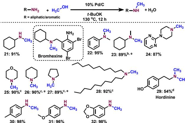
**Scheme 5.** Pd/C-catalyzed *N*-methylation of amines with MeOH.<sup>[a]</sup> Reaction conditions: 0.5 mmol of amine, 10% Pd/C (4.7 mol% Pd, 25 mg), 2 ml of MeOH as a reagent and solvent, *t*-BuOK (1 mmol, 2 equiv.), 12 h, 130 °C, isolated yields. <sup>b</sup> 14 h. <sup>c</sup> 16 h. <sup>d</sup> 30 h. <sup>e</sup> GC yields.
