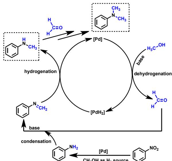
**Figure 2.** Plausible reaction mechanism for Pd/C-catalyzed *N*-methylation of nitroarenes
