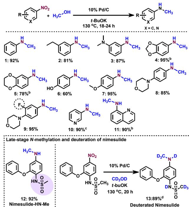
**Scheme 2.** Pd/C-catalyzed *N*-methylation of nitroaromatics with MeOH.<sup>[a]</sup>
