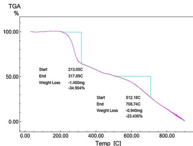
Fig. 1 Thermogravimetric curve of SB-1
