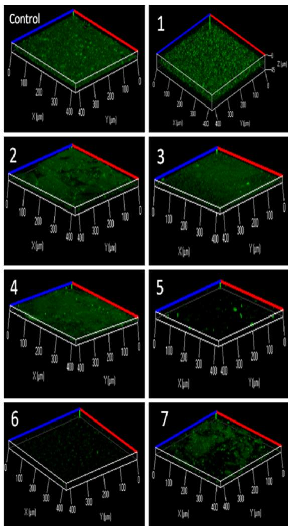
**Fig. 6** Confocal laser scanning microscope analysis of biofilm. *Pseudomonas aeruginosa* shows the patches of fluorescence in presence of Schiff bases, SB-5, SB-6 and SB-7, indicated a truncated formation of biofilm. However, in absence of Schiff bases (control), fluorescence was regular and entire, thus indicating an intact biofilm
