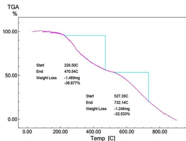
**Fig. 2** Thermogravimetric curve of SB-5
