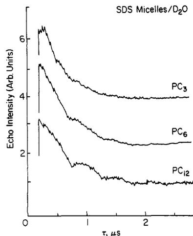
Figure 2. Two-pulse ESE signals at 4.2 K of photoionized  $\text{PC}_3$ ,  $\text{PC}_6$ , and  $\text{PC}_{12}$ , solubilized in sodium dodecyl sulfate micelles. The signals are offset vertically.
