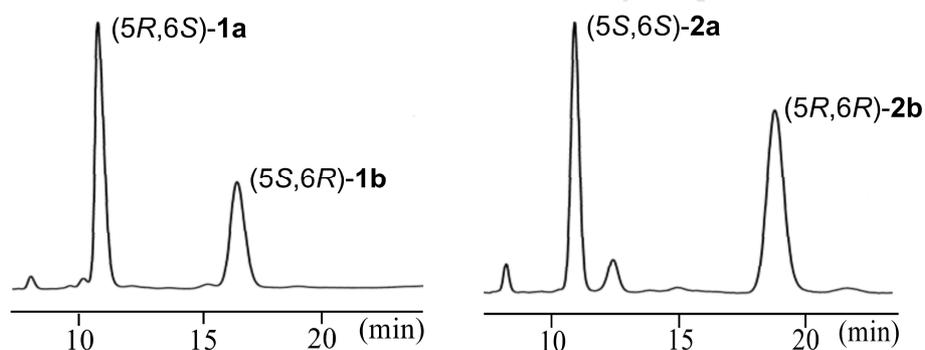
**Fig. 3.** HPLC elution profiles of lycopene-5,6-diol stereoisomers (**1a,b**) and (**2a,b**). Column: CHIRALPAK AD-H (daicel)  $0.46 \times 25$  cm; eluent: 2-PrOH-hexane (15:85); flow rate: 1.0 mL/min; temperature: 25 °C; detection: 450 nm.
