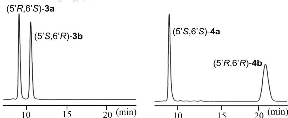
**Fig. 4.** HPLC elution profiles of  $\gamma$ -carotene-5',6'-diol stereoisomers (**3a,b**) and (**4a,b**). Column: CHIRALPAK AD-H (daicel)  $0.46 \times 25$  cm; eluent: 2-PrOH-hexane (15:85); flow rate: 0.6 mL/min; temperature: 25 °C; detection: 450 nm.
