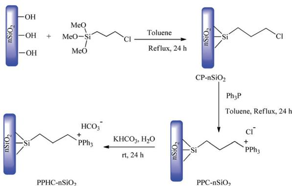
Scheme 2 Synthesis of propylphosphonium hydrogen carbonate ionic liquid supported on nano-silica (PPHC-*n*SiO<sub>2</sub>).
