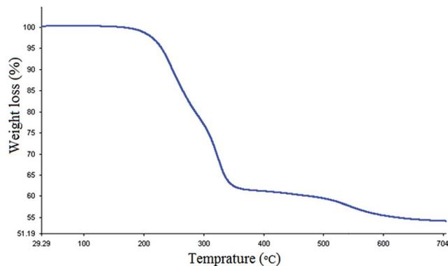
Fig. 2 TGA curve of PPHC-*n*SiO<sub>2</sub> catalyst.
