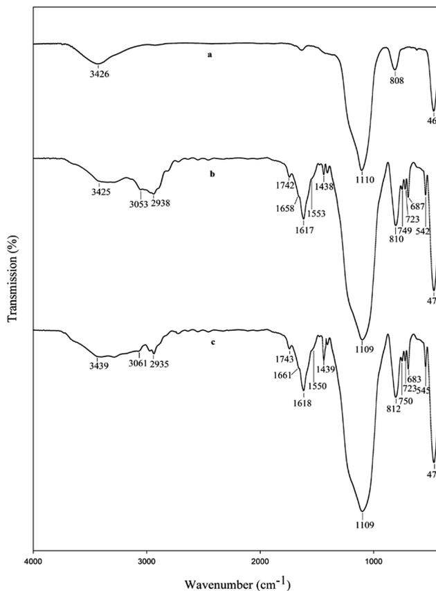
Fig. 1 FT-IR spectra of: (a) nano-SiO<sub>2</sub>; (b) PPHC-*n*SiO<sub>2</sub> and (c) the 5-times reused catalyst.
