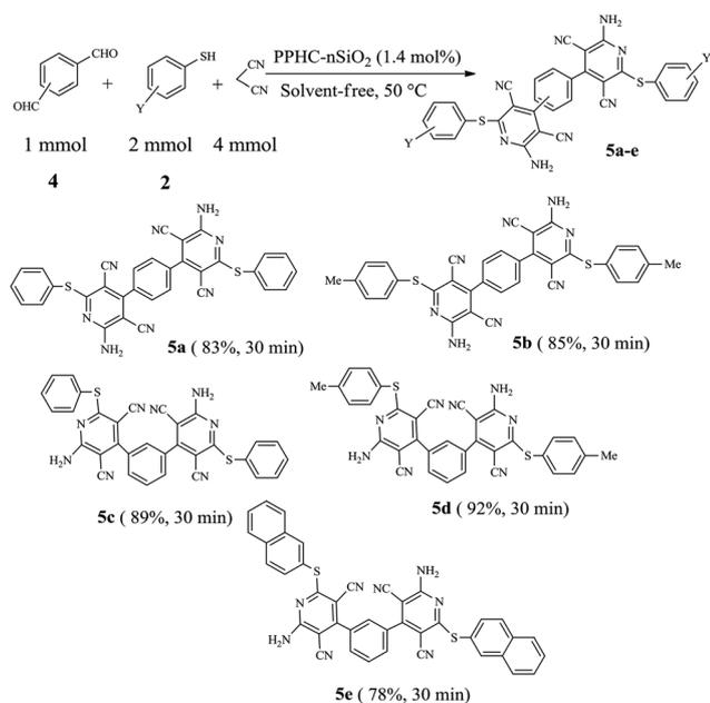
Scheme 3 Synthesis of bis-pyridines from dialdehydes catalyzed by PPHC-*n*SiO<sub>2</sub>.
