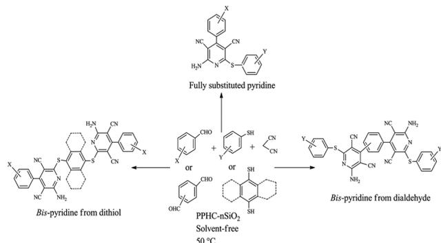
Scheme 1 Synthesis of fully substituted pyridines and bis-pyridines catalyzed by PPHC-*n*SiO<sub>2</sub>.
