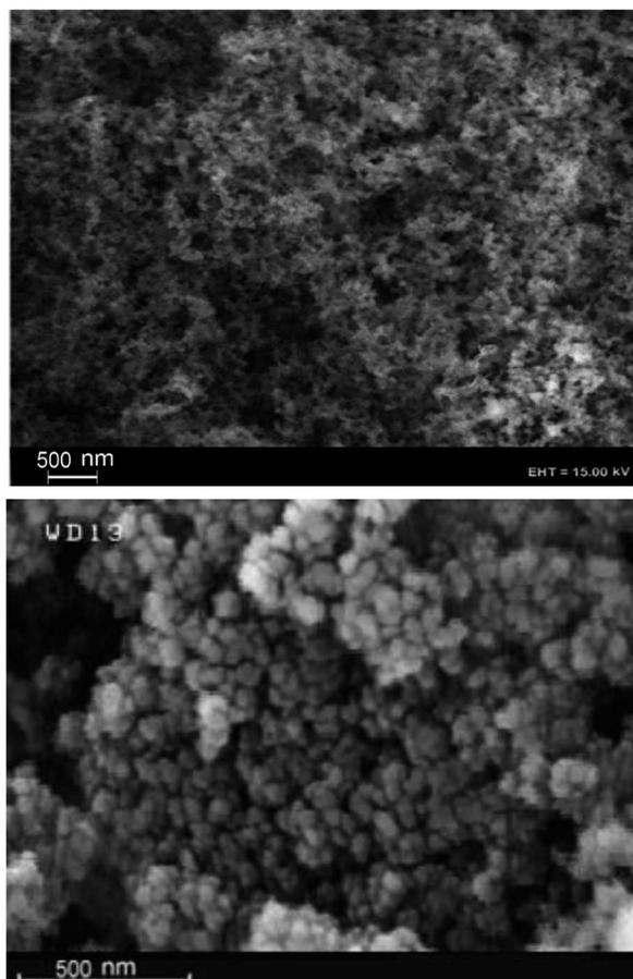
Fig. 3 SEM images of: (a) nano-silica and (b) PPHC-*n*SiO<sub>2</sub> catalyst.
