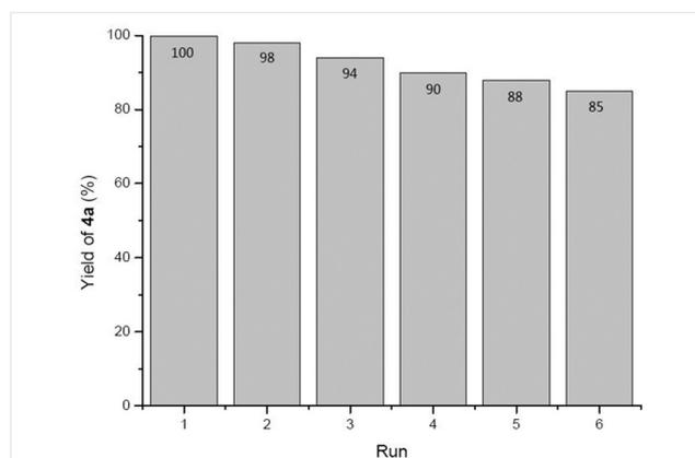
**Figure 2** Recycling of the catalyst [DABCO-H][AcO] for the synthesis of **4a**. Reagents and conditions: isatin (**1a**, 5 mmol), malononitrile (**2a**, 5 mmol), diethyl phosphite (**3a**, 5 mmol), catalyst (7 mol%), THF (2 mL), r.t.
