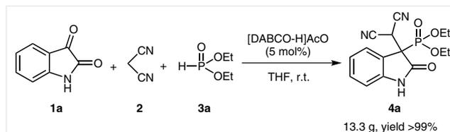
**Scheme 4** Synthesis of 2-oxindol-3-ylphosphonate **4a** on 40-mmol scale
