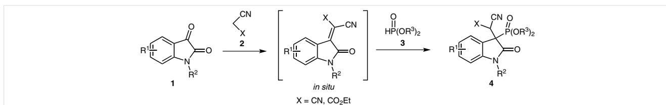
**Scheme 1** Tandem reaction for the one-pot synthesis of 2-oxindol-3-ylphosphonates **4**
