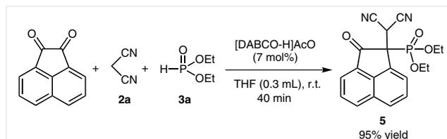
**Scheme 3** Reaction of acenaphthenequinone with malononitrile and diethyl phosphite
