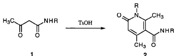
Reaction of *N*-propyl-3-oxobutanamide (**1b**) was performed by use of an equimolar amount of *p*-toluenesulfonic acid as a catalyst. When the reaction was performed using a solvent, 4,6-dimethyl-1-propyl-5-(propylaminocarbonyl)-2-pyridone (**2b**) was obtained in moderate yield (for example, benzene: 46%, acetonitrile, 45%, dichloromethane: 14%), while **2b** was obtained in 84% yield when the reaction was performed without solvent at 100–110°C for 11 hours. The reaction proceeded
