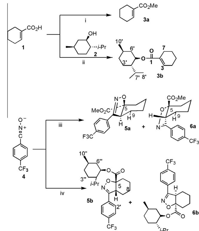
**Scheme 1.** Cycloaddition of dipole **4** to dipolarophiles **3a,b**. i MeOH,  $\text{H}^+$ , ii DCC, DMAP, iii **3a**,  $\text{CH}_2\text{Cl}_2$ ,  $\text{Yb}(\text{OTf})_3$ -ligand A (Fig. 1) or  $\text{Yb}(\text{OTf})_3$ -ligand B or without the catalyst, iv **3b**,  $\text{CH}_2\text{Cl}_2$ ,  $\text{Yb}(\text{OTf})_3$ -rac ligand B or without the catalyst.
