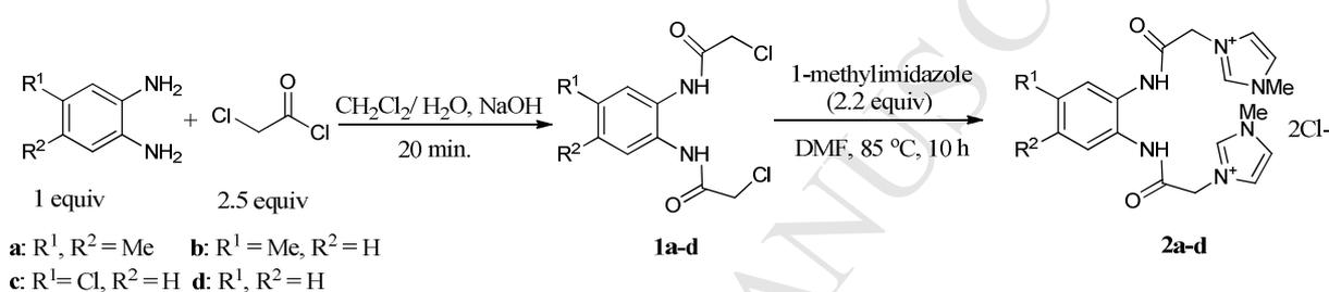
**Scheme 2.** Synthetic route for preparation of bis-imidazole ligand precursor
