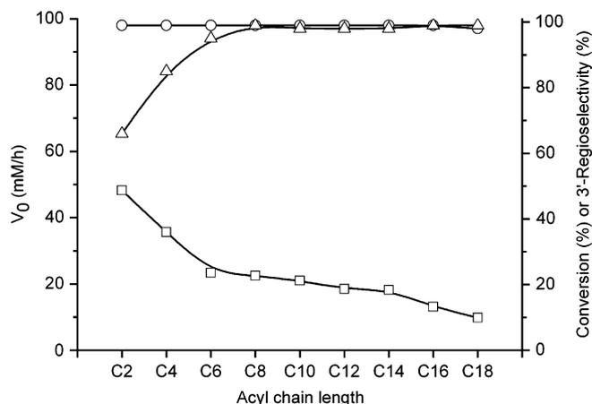
**Figure 1.** Effect of acyl chain length on PSL-C-catalyzed acylation of FUDr. The reaction was carried out at 40 °C, 250 rpm by adding 40 U PSL-C into anhydrous THF (2 mL) containing FUDr (0.04 mmol), vinyl esters (0.16 mmol) with [C<sub>4</sub>MIM]PF<sub>6</sub> (10 mg) as the additive. Symbols: V<sub>0</sub> (□); conversion (○); 3'-regioselectivity (△).
