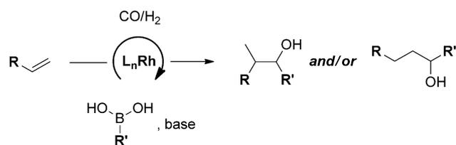
**Scheme 1.** Single Rh(I)/L catalyst for tandem hydroformylation/arylation reaction.
