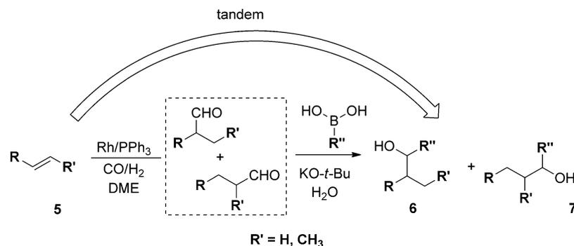
**Scheme 2.** Transformation of olefins into secondary alcohols using Rh(I)/PPh<sub>3</sub> a multicatalytic tandem hydroformylation/arylation reaction.
