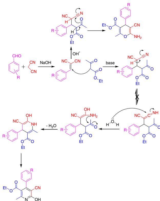
**Mechanism 1.** Plausible reaction mechanism for the synthesis of tetra-substituted 4*H*-pyrans.
