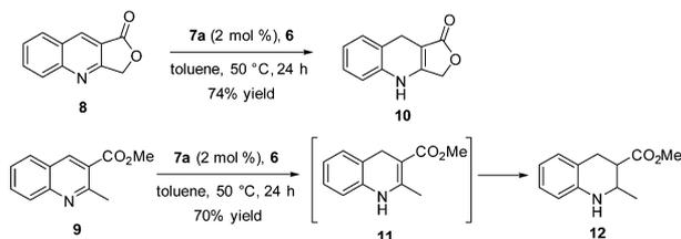
Whereas the formation of the dihydroadducts **10** and **11** was expected in both the cases, ester derivative **9** underwent a complete reduction furnishing the tetrahydroquinoline **12** in 70% yield.
