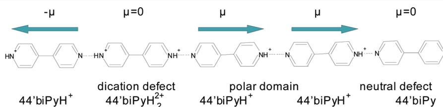
Figure 5. Chain interval of NH<sup>+</sup>...N-bonded disproportionated 44'biPyH<sup>+</sup> cations, 44'biPyH<sub>2</sub><sup>2+</sup> dications, and 44'biPy molecules. 44'biPy molecules and 44'biPyH<sub>2</sub><sup>2+</sup> dications separate the chain fragments of opposite polarization, depending on the H<sup>+</sup> position in the hydrogen bonds.
