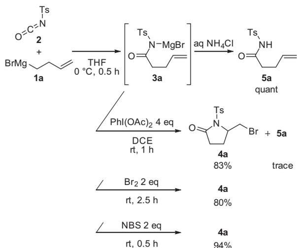
**Scheme 1.** Tandem carbamoylation–oxidative bromolactamization of 3-butenylmagnesium bromide **1a** with isocyanate **2**.
