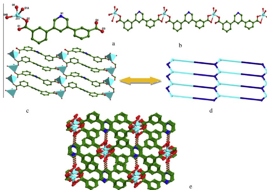
**Fig. 1.** (a) Coordination environments of the Zn<sup>II</sup> ions in **1**. Hydrogen atoms and free water molecule are omitted for clarity; (b) the infinite 1D chain formed by Zn<sup>II</sup> ions and pddb<sup>2-</sup> ligand. (c) polyhedral view of the 2D layer in **1**; (d) The 3,3-connected topology of the 2D layer viewed by *b* axis; (e) Perspective view of the supermolecular framework through two kinds of hydrogen-bonding interaction.
