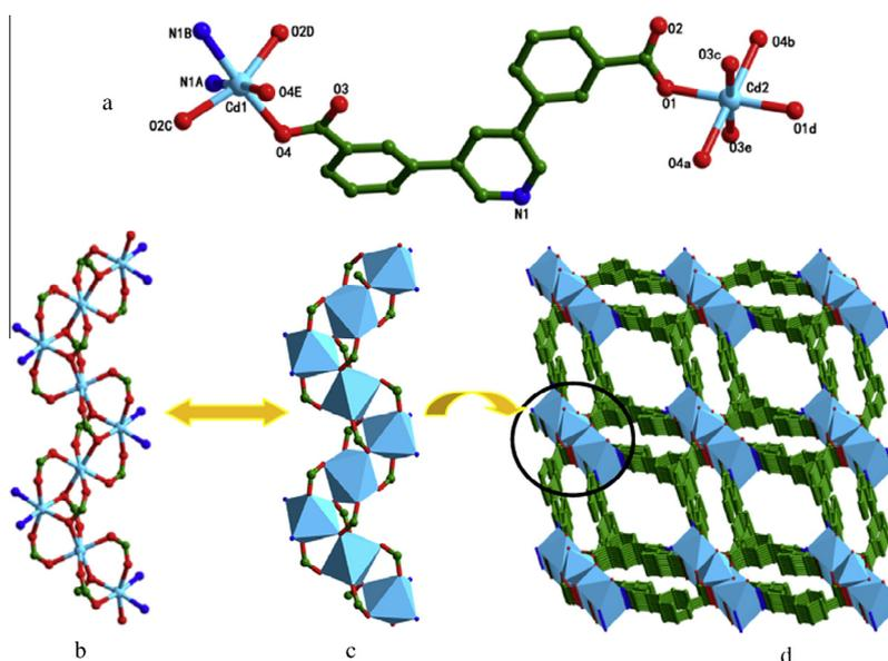
**Fig. 3.** (a) Coordination environments of the Cd<sup>II</sup> ions in **3**. (b) The rod SBU unit formed by Cd<sup>II</sup> ions and carboxylate groups from the pddb<sup>2-</sup> ligand. (c) polyhydral view of the rod SBU in **3**; (d) Perspective view of the 3D framework formed by the rod SBU linking with four neighbor SBU units by pddb<sup>2-</sup> ligand. Hydrogen atoms and free water molecule are omitted for clarity.
