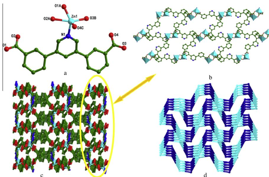
**Fig. 2.** (a) Coordination environments of the Zn<sup>II</sup> ions in **2**. (b) Perspective view of the 2D layer in **2**. (c) Perspective view of the 3D framework extended by Zn<sup>II</sup> coordinating with nitrogen atoms, viewed by the *c* axis. (d) The 3,6-connected topology of the 3D framework. Hydrogen atoms and free water molecule are omitted for clarity.
