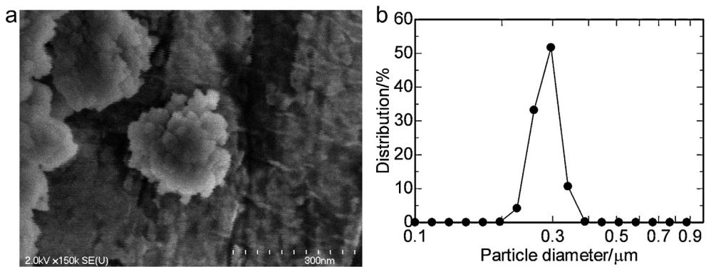
**Fig. 1.** ZSM-5 nanoparticles. (a) FE-SEM image and (b) particle size distribution.
