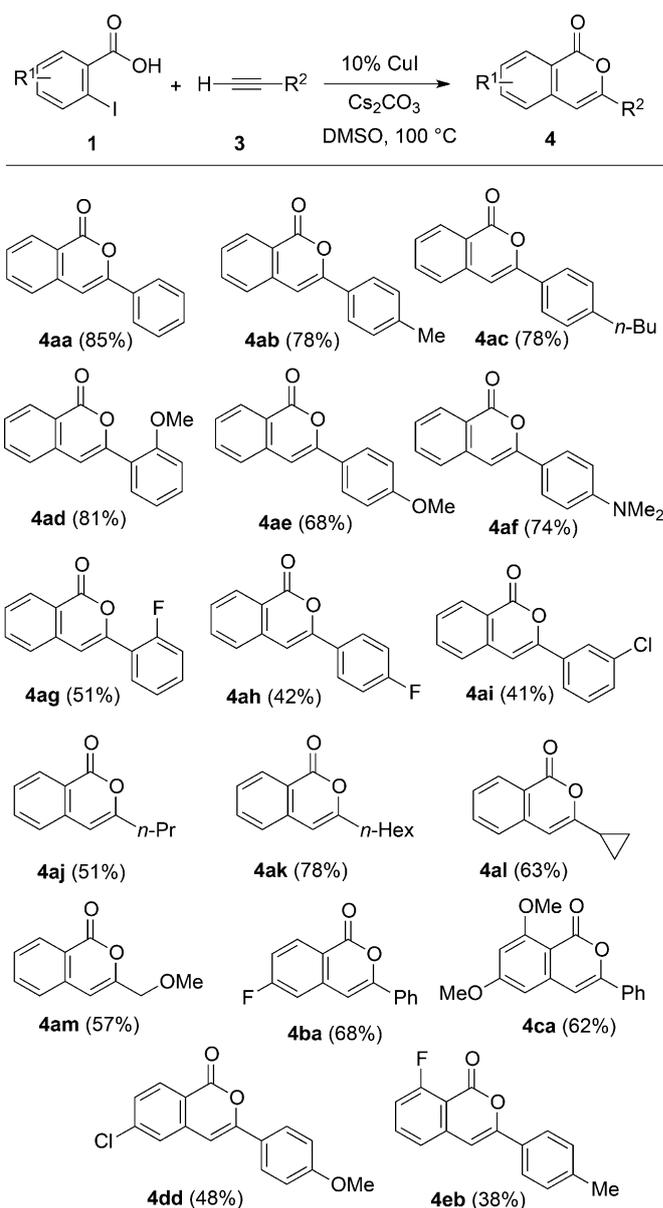
**Scheme 2.** Synthesis of isocoumarins from the coupling reactions of 2-iodobenzoic acids and terminal alkynes. *Reaction conditions:* **1** (2.0 mmol), **3** (2.2 mmol), CuI (0.2 mmol) and  $\text{Cs}_2\text{CO}_3$  (4.0 mmol) at 100 °C for 12 h.
