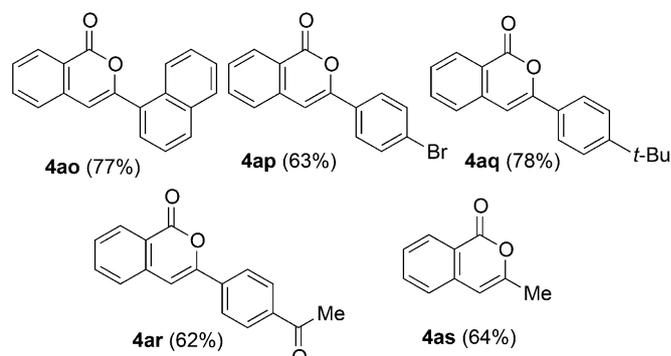
**Scheme 4.** Synthesis of isocoumarins from the coupling reactions of 2-iodobenzoic acids and alkynyl carboxylic acids. *Reaction conditions:* **1** (2.0 mmol), **2** (2.2 mmol), CuI (0.2 mmol) and Cs<sub>2</sub>CO<sub>3</sub> (4.0 mmol) at 100 °C for 12 h.
