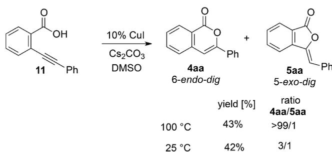
**Scheme 6.** Cyclization of 2-(phenylethynyl)benzoic acid under this catalytic system.
