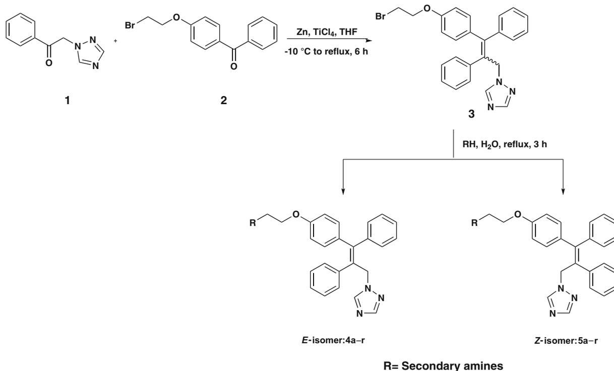
**Scheme 3** Synthesis of tamoxifen containing 1,2,4-triazole and its side chain analogs. Compounds **4a–r** are presented as *E*-isomers and compounds **5a–r** are presented as *Z*-isomers
