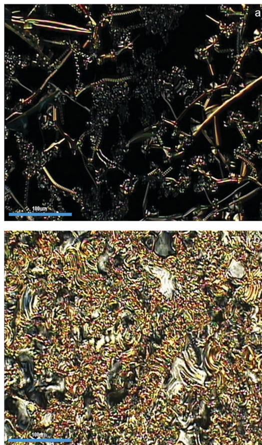
Fig. 4 Optical photomicrographs (crossed polarizers along the edges) of a 5 μm thick film with planar anchoring of compound IIIc : (a) T = 162 °C: formation of helical filaments and beaded filaments characteristic of a B7 phase; (b) T = 145 °C: crystal phase.
