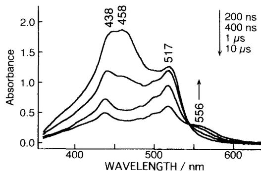
Fig. 3. Transient absorption spectra of 2-chlorophenothiazine in deoxygenated methanol: measured at 200, 400 ns, 1 and 10  $\mu$ s after UV (308 nm) excitation. Concentration is  $5.0 \times 10^{-4}$  mol dm $^{-3}$ .
