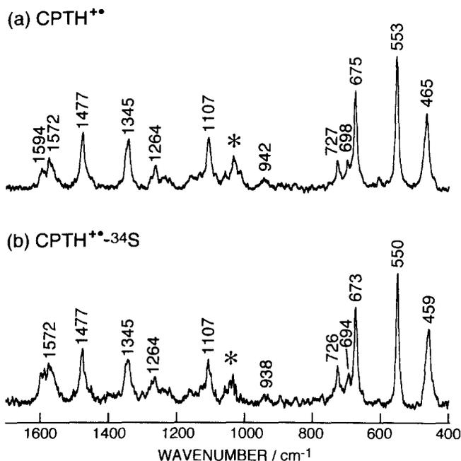
Fig. 10. Transient resonance Raman spectra of the cation radical of 2-chlorophenothiazine and its  $^{34}\text{S}$  substituted analogue in methanol: (a)  $\text{CPTH}^+$  normal species; (b)  $\text{CPTH}^+-^{34}\text{S}$ . Pump wavelength: 308 nm and probe wavelength is 517 nm. Concentration is  $2.0 \times 10^{-3} \text{ mol dm}^{-3}$ . The asterisk (\*) denotes solvent bands.
