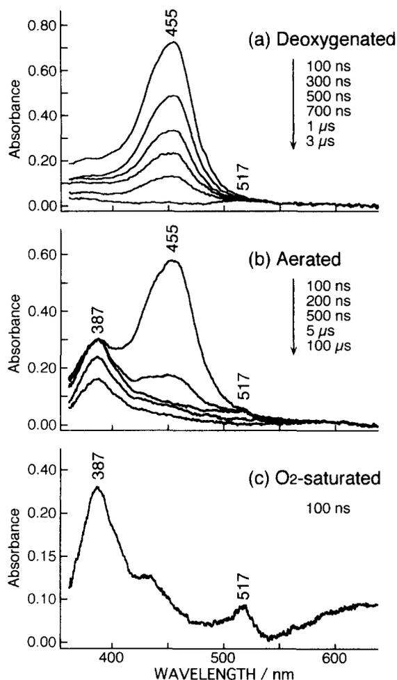
Fig. 2. Transient absorption spectra of phenothiazine: (a) in deoxygenated methanol measured at 100, 300, 500, 700 ns, 1 and 3  $\mu$ s after excitation with UV (308 nm) light; (b) in aerated methanol measured at 100, 200, 500 ns, 5 and 100  $\mu$ s; (c) in oxygenated methanol measured at 100 ns. Concentration is  $1.0 \times 10^{-3}$  mol dm $^{-3}$ .
