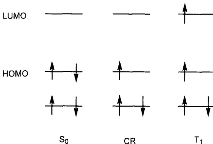
Fig. 11. Electronic configurations of the  $T_1$  state and cation radical.
