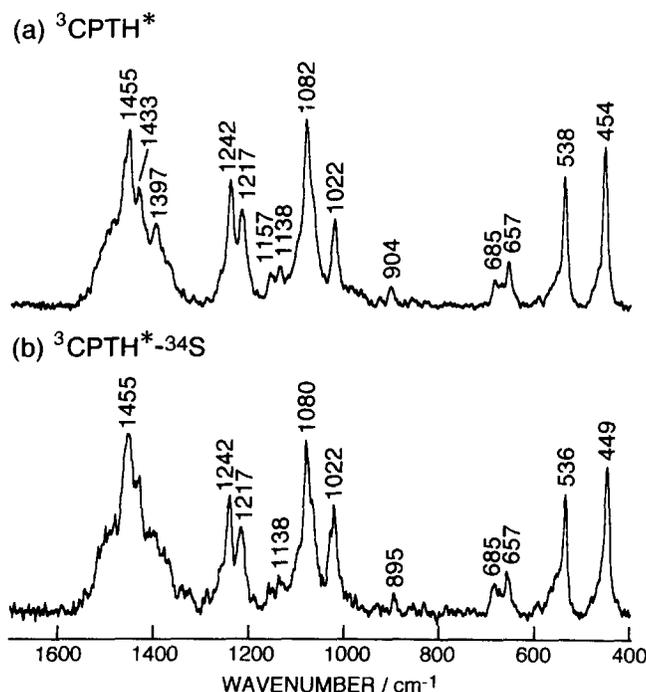
Fig. 8. Transient resonance Raman spectra of the  $T_1$  state of 2-chlorophenothiazine and its  $^{34}\text{S}$  substituted analogue in deoxygenated methanol: (a)  $^3\text{CPTH}^*$  normal species; (b)  $^3\text{CPTH}^*-\text{}^{34}\text{S}$ . Pump wavelength: 308 nm and probe wavelength is 456 nm. Concentration:  $2.0 \times 10^{-3} \text{ mol dm}^{-3}$ .
