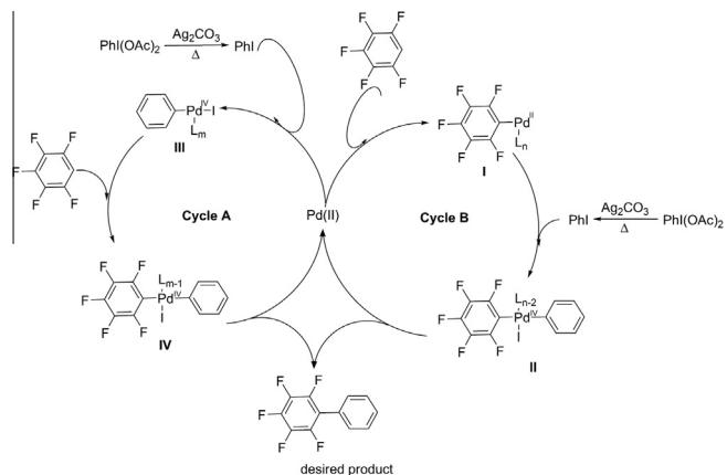
**Scheme 1.** Two assumed mechanisms of the transformation.**Table 3**Pd-catalyzed direct arylation of pentafluorobenzene with (diacetoxyiodo)benzene derivatives<sup>a</sup>
