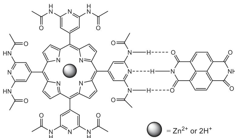
**Figure 1.** Structure of the rigid coplanar dyad, assembled by three-point hydrogen bonding which may mediate electron transfer processes, can be formed by mixing 5,10,15,20-Tetrakis(3,5-diacetamido-4-pyridyl)porphyrin (**1**) and naphthalene diimide (NDI) in different aprotic solvents.
