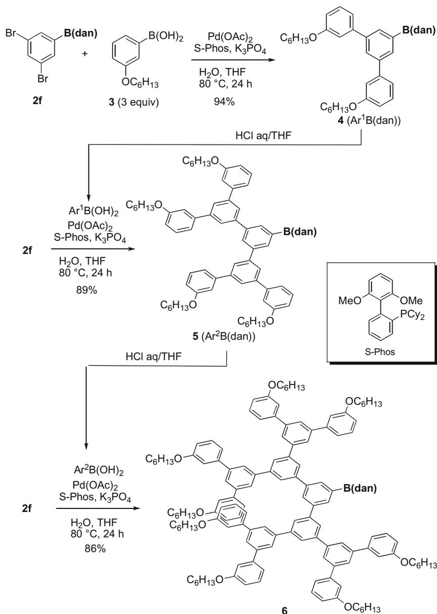
**Scheme 1.** Iterative synthesis of building blocks for the convergent dendrimer synthesis using **2f** as the cross-coupling module.
