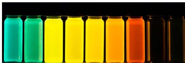
**Figure 7.** Fluorescence of compound **4p** with variable solvent polarity (from left to right: *n*-pentane, cyclohexane, toluene, 1,4-dioxane, diethylether, ethyl acetate, dichloromethane, *N,N*-dimethyl formamide, acetonitrile;  $\lambda_{ex} = 365$  nm, hand-held UV lamp).
