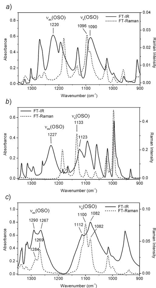
**Fig. 6** Vibrational spectra in the OSO stretching region of: (a) [Ti<sub>2</sub>Cl<sub>8</sub>(μ-sulfolane-*O,O'*)<sub>2</sub>] (**1d**), (b) [ZrCl<sub>4</sub>(μ-Ph<sub>2</sub>SO<sub>2</sub>-*O,O'*)<sub>2</sub>] (**2c**), (c) ZrCl<sub>4</sub>(Me<sub>2</sub>SO<sub>2</sub>)<sub>2</sub> (**2aa**).
