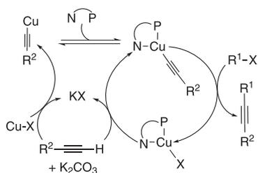
**Scheme 3.** Supposed mechanism for the Sonogashira reaction catalyzed by **L1/L2** and Cu(I) *in situ*.
