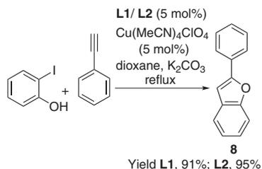
**Scheme 4.** The reaction between *o*-iodophenol and phenylacetylene.
