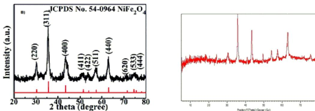
Figure 3. The XRD patterns of a) NiFe<sub>2</sub>O<sub>4</sub>@SiO<sub>2</sub>@aminoglucose and b) NiFe<sub>2</sub>O<sub>4</sub>
