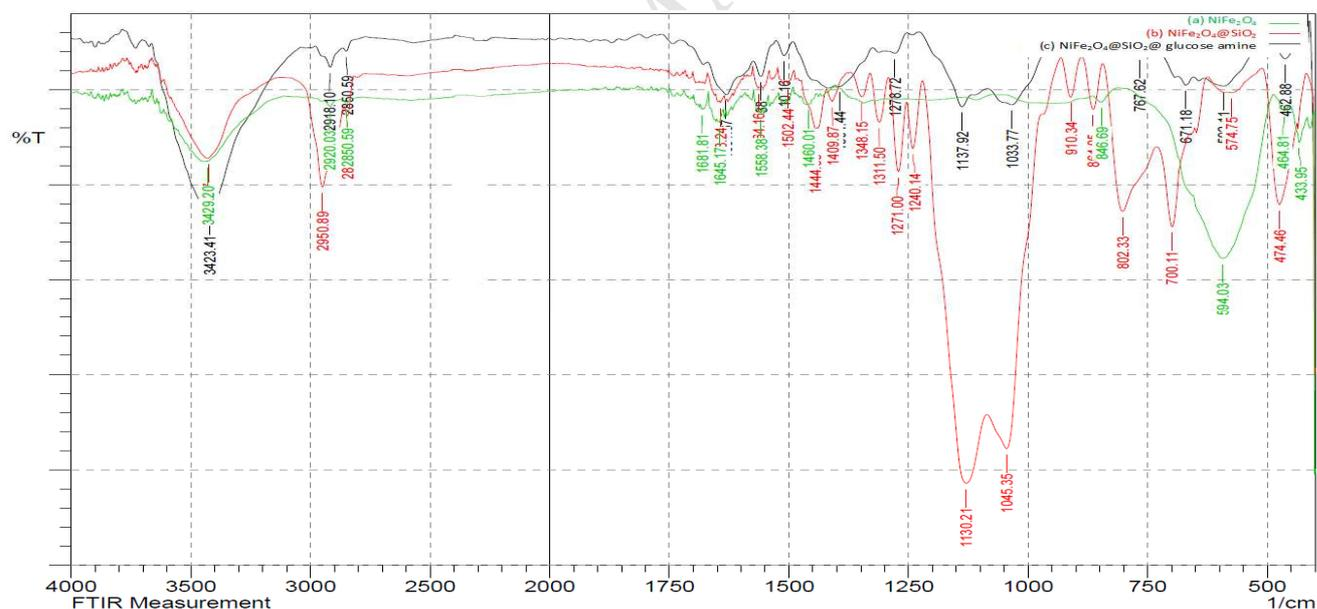
Figure 1. FT-IR spectra of (a)  $\text{NiFe}_2\text{O}_4$ , (b)  $\text{NiFe}_2\text{O}_4@\text{SiO}_2$ , (c)  $\text{NiFe}_2\text{O}_4@\text{SiO}_2@\text{aminoglucose}$  MNPs
