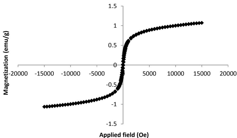
Figure 6. Vibrating scanning magnetometry (VSM) curve of the synthesized nanocatalyst
