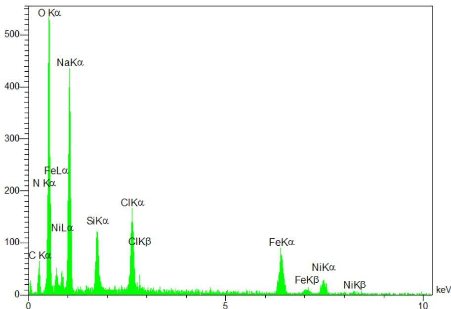
Figure 4. EDX results of the synthesized  $\text{NiFe}_2\text{O}_4@\text{SiO}_2@\text{aminoglucose}$  MNPs
