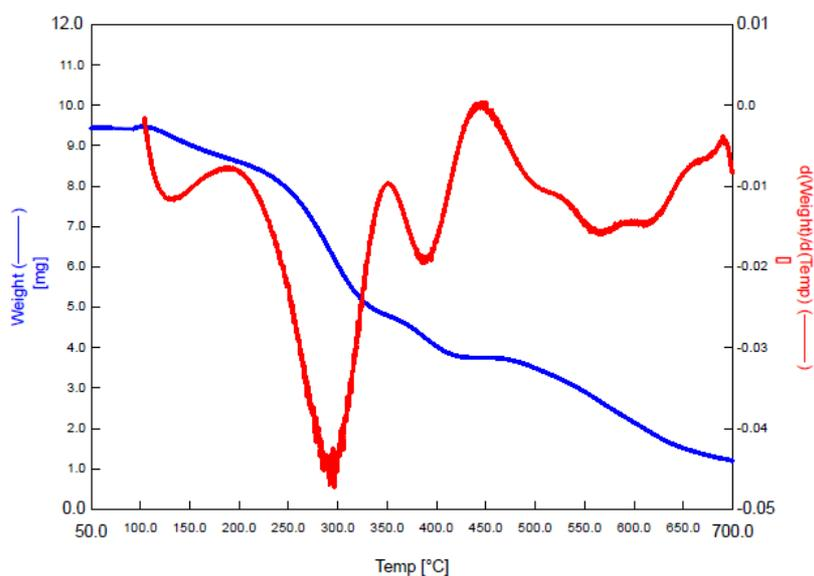
Figure 5. Thermogram of TGA (blue colour) and DTG (red colour) analysis of the synthesized  $\text{NiFe}_2\text{O}_4@ \text{SiO}_2@$  aminoglucose MNPs.
