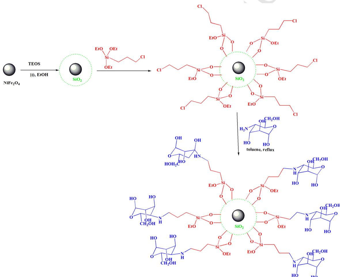
Scheme 1. Stepwise synthesis pathway of  $\text{NiFe}_2\text{O}_4@\text{SiO}_2@\text{glucoseamine}$
