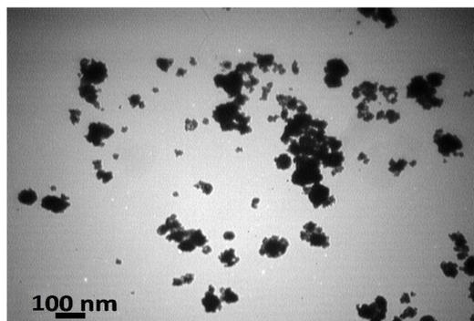
Figure 2. The TEM image of synthesized NiFe<sub>2</sub>O<sub>4</sub>@SiO<sub>2</sub>@aminoglucose
