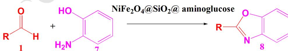
Scheme 6. Synthesis of benzoxazoles using NiFe<sub>2</sub>O<sub>4</sub>@SiO<sub>2</sub>@ aminoglucose
