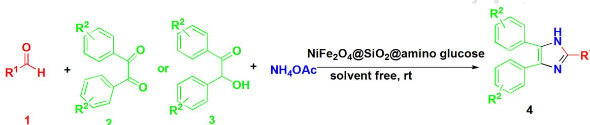
Scheme 2. Synthesis of trisubstituted imidazoles using  $\text{NiFe}_2\text{O}_4@\text{SiO}_2@\text{amino glucose}$
