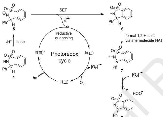
**Scheme 3.** Proposed mechanism of the photocatalyzed aerobic oxidation
